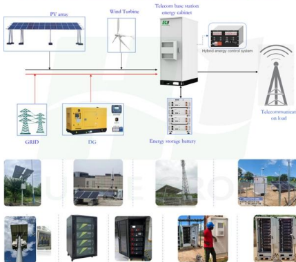
Base station energy composition diagram
